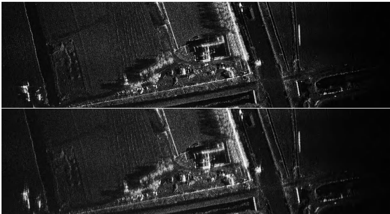
Figure 18: Full-resolution SAR (top) and CommSAR (bottom) imaging results for Flight #2 (512-symbol modulation).
