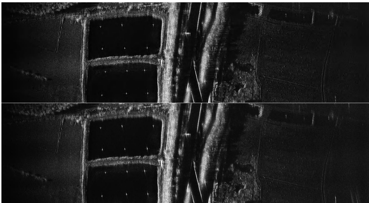
Figure 19: Full-resolution SAR (top) and CommSAR (bottom) imaging results for Flight #3 (1024-symbol modulation).
